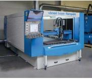
KOMPAKT Laser with the manually extendable grid is designed for 1,500  $\times$  3,000 mm sheets. Laser machines have been manufactured by Vanad since 2012 for the smallest sheet sizes of 1,500  $\times$  3,000 mm, biggest size 2,000  $\times$  6,000 mm with a maximum performance of 3 kW.
