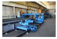
The Vanad PROXIMA machine with an additional RotCUT equipment for tubes and profiles cutting.
