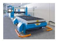
Vanad KOMPAKT Laser with two exchangeable material grids.
