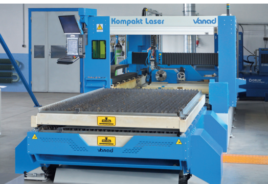
▲ Vanad KOMPACT Laser with two hydraulically exchangeable material grids and 2kW IPG laser source, installed in 2016
