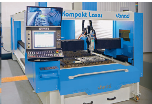
▲ Vanad KOMPACT Laser with a manually exchangeable material grid and 3kW IPG laser source, installed in 2017
