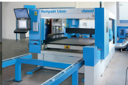
▲ Vanad KOMPACT Laser with a motor-powered extendable material grid and 1kW IPG laser source, installed in 2017
