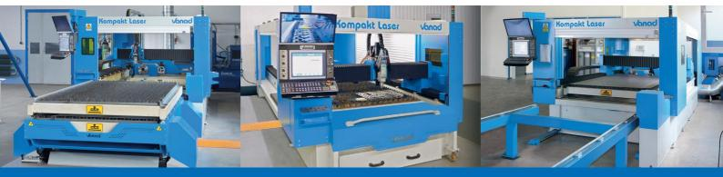
Vanad KOMPAKT Laser with two hydraulically exchangeable material grids and 2kW IPG laser source, installed in 2016 Vanad KOMPAKT Laser with a manually exchangeable material grid and 3kW IPG laser source, installed in 2017
