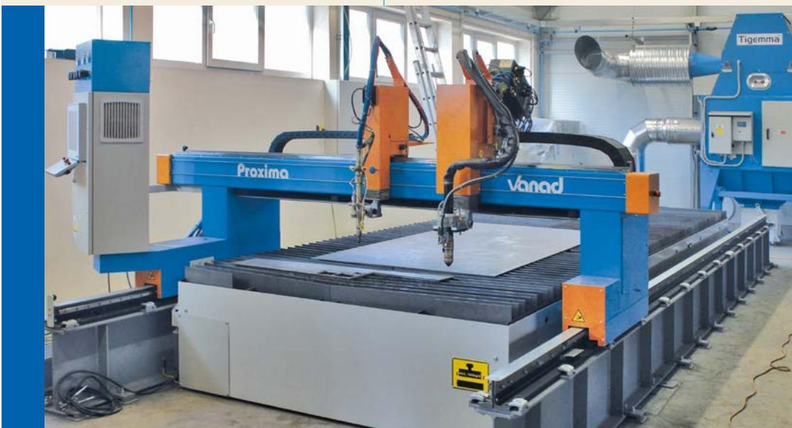
◀ Comprehensive cutting station PROXIMA built in 2014. CNC cutting machine is equipped with the Kjellberg HiFocus 360i plasma system, oxy-fuel technology, Tigemma filter system and Orlik compressor
