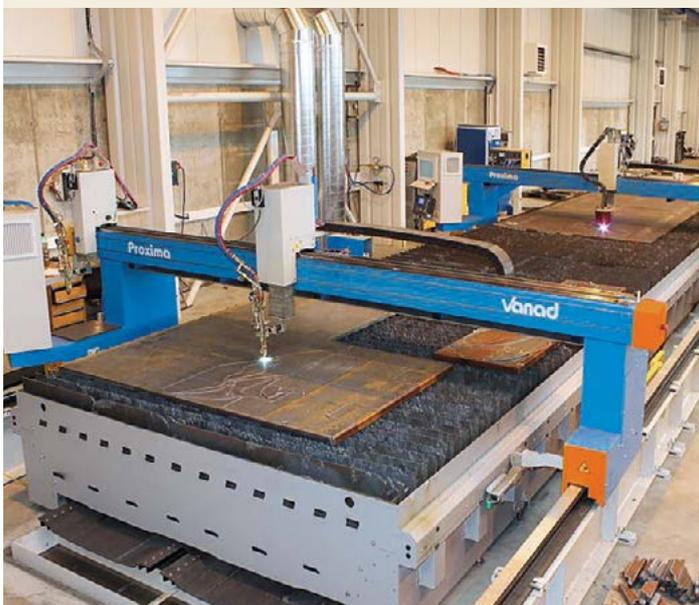
▶ Semi-automatic three-torch head is an optional device used for direct cutting of the material used for bevel cutting of materials. Created bevels are often used for subsequent welding
