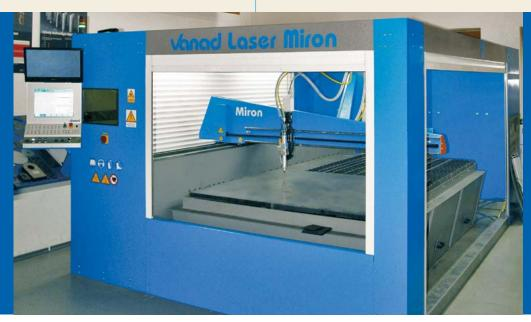
◀ MIRON Laser is an efficient CNC cutting machine equipped with fiber laser, which effortlessly cuts metal and non-metal materials such as mica plates, HSS sheets, klingerit, mirelon, polyethylene foam, antivibration rubber sheets, cardboard, cork, brass, bronze, copper and tar paper.
