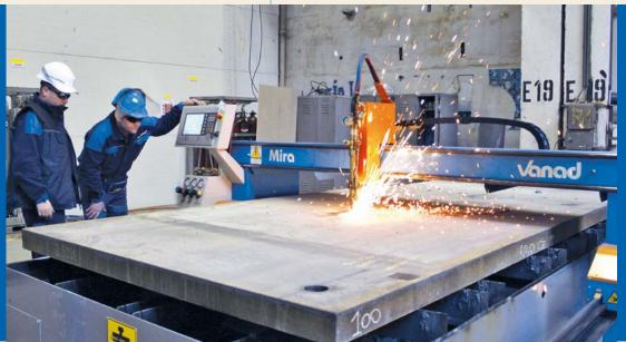
■ The CNC cutting machine Vanad MIRA is equipped with oxy-fuel technology, laser pointer and electric flame ignition of the oxy-fuel torch. The picture shows the piercing of 100 mm structural steel.
