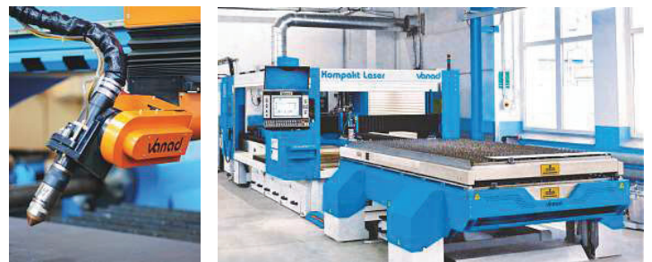
The Vanad Bluester machine (left) is used for heavy operations and allows cutting of material of thickness up to 400mm; Right: The Vanad Kompakt Laser
